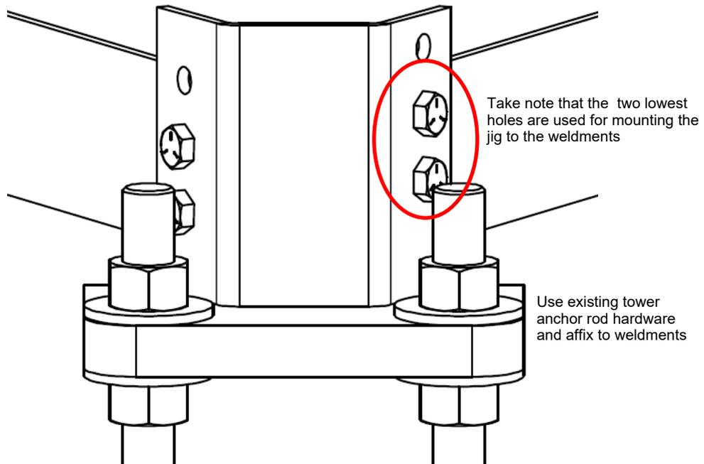
Anchor rod plate. Use 1" nuts attached to plate at bottom of anchors.
