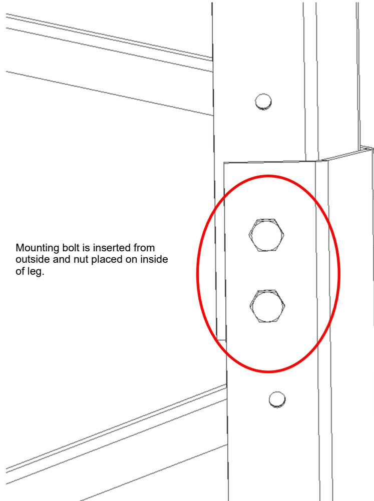
Mounting bolt is inserted from outside and nut placed on inside of leg.
