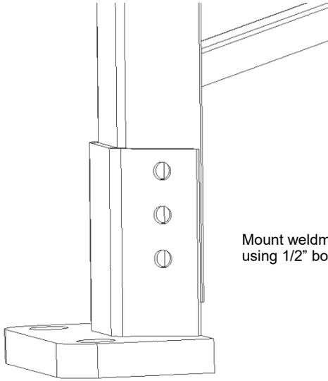
Mount weldments to bottom section using 1/2" bolts supplied, 6 bolts per leg.
