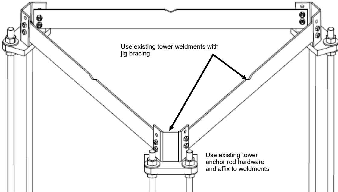
Take note of hole offset on jig bracing and notch. Left side has holes offset higher and the notch is on top.
